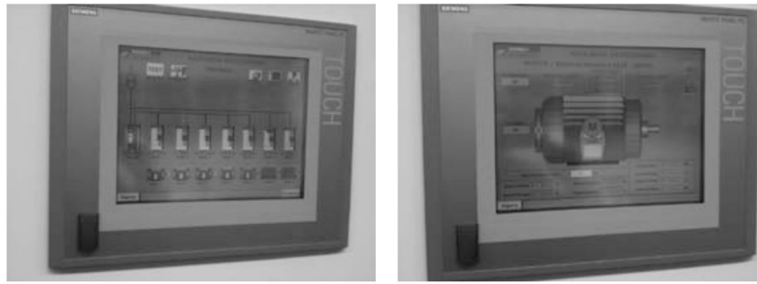
Fig.10. a,b "D.A. Large Drives" OP touch-screen troubleshooting system tool overview, screenshots
